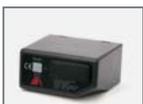
P111274 - RME Single-channel metal detector with installation base. Power supply 24Vac. Power supply LED. Channel LED. Pulse on release configuration. Presence relay with pulse or continuous operation. Pulse relay with deactivation possibility.
